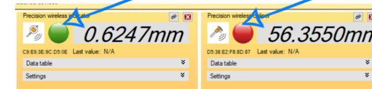
Select Filtering device mode in Connection menu to view only MICROTECH instruments in Available devices area
