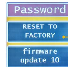
Push 10 times to RESET device to factory settings
